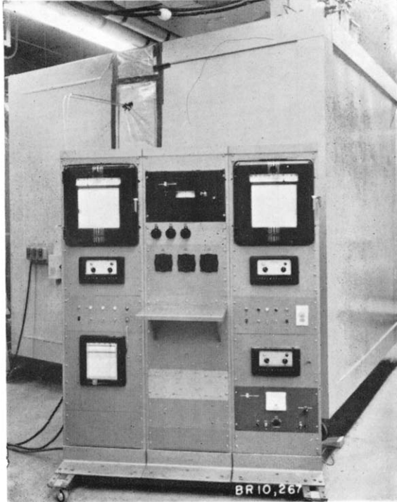
FIG. 2. Test unit showing temperature control panel and measuring and recording instruments.
